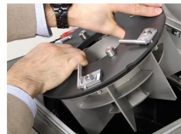
changing and cleaning the contaminant container.
