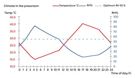
The relative humidity of an area is directly dependent on the air temperature. The physical law shown here is quite simple: rising air temperature leads to decreasing relative humidity and vice versa. Fluctuating ambient conditions have a notable negative impact on the printing papers.
