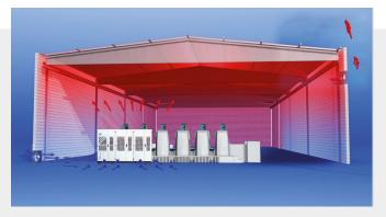
Air-cooled peripheral units discharge this hot waste air directly into the printing room. An apparently easy and inexpensive solution that however causes severe changes of the room climate.
