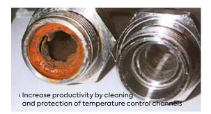
The moldclean series was designed to clean scaled cooling channels of injection moulds and heat exchanger systems. The ph-value control and the flow rate measurement indicate the progress of the cleaning process.
