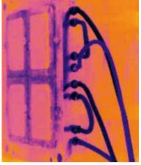
Homogenous temperature distribution in the injection mould after the temperature conditioning circuits have been cleaned
