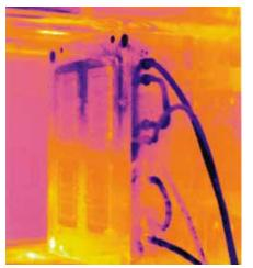
Inhomogeneous temperature distribution in the injection mould due to polluted temperature conditioning circuits.
